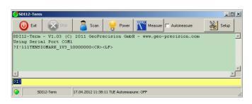
The most important SDI12 commands (letters a and b are for SDI addresses (0..9, a-z, A-Z, the question mark stands for "unknown" and works only, if only one sensor is connected to the SDI 12 bus, if several sensors are connected, it can not be used.):
